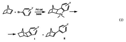
The palladacycle complex, which also is a key intermediate in other syntheses involving palladium(IV) [3], could be trapped with a stabilizing ligand such as phenanthroline in a stoichiometric reaction according to eq. 2 [4]. The synthesis requires palladium exchange with arylmercury halides followed by norbornene insertion [5] and cyclization [4] in the presence of suitable ligands.
